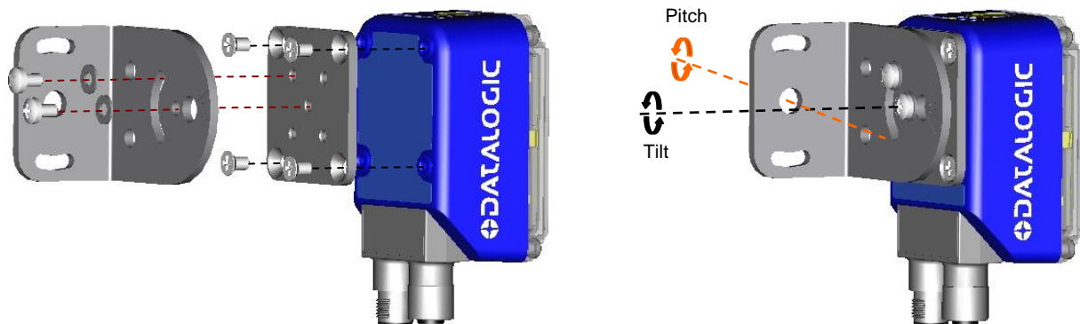
Figure 2 – Positioning with Mounting Bracket
