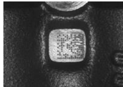
Dot Peening On Scratched Surface
