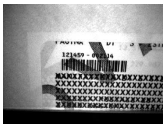
Figure 17 - Overprinted Barcode Readable by Matrix 210™ also Through the Envelope Window Film
