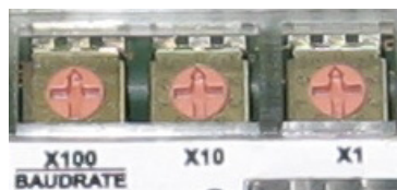
Figure 12 – Address Selection Switches
