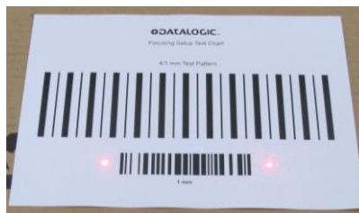
Figure 8 –Aligning the Focusing and PPI Setup Chart Using Laser Pointers as Reference
